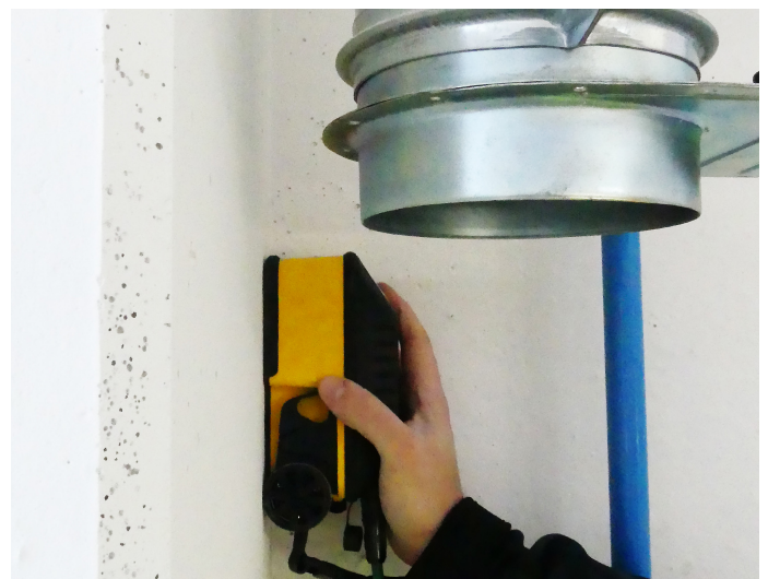
C-thru XS's compact size and light weight allow to easily investigate hard to reach areas and around obstructions.
