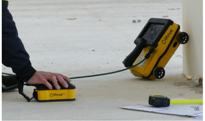
C-thruve XS can be connected via LAN to the C-thruve device allowing for a real-time visualization of the collected data on the multi-touch display.
