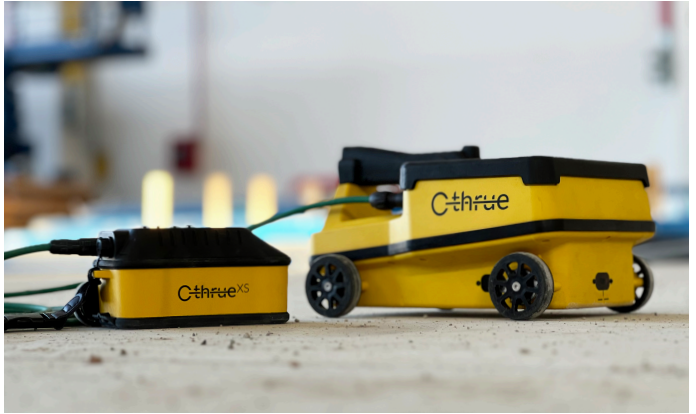
To survey hard to reach areas, C-thru can be connected to the C-thru XS device and easily reach inaccessible spots.
